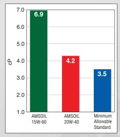
The High-Temperature/High-Shear Viscosity Test (ASTM D5481) measures a lubricant's viscosity under severe high-temperature and shear conditions, similar to severe operating conditions experienced by motorcycles. Higher values indicate improved wear protection.
